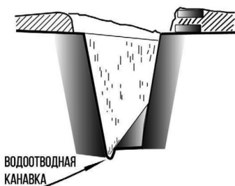
Rice. 2. Drainage groove on trench bottom
